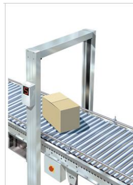
Profile scanner (source http://www.itsuk.org.uk/volume_and_weight.php )
