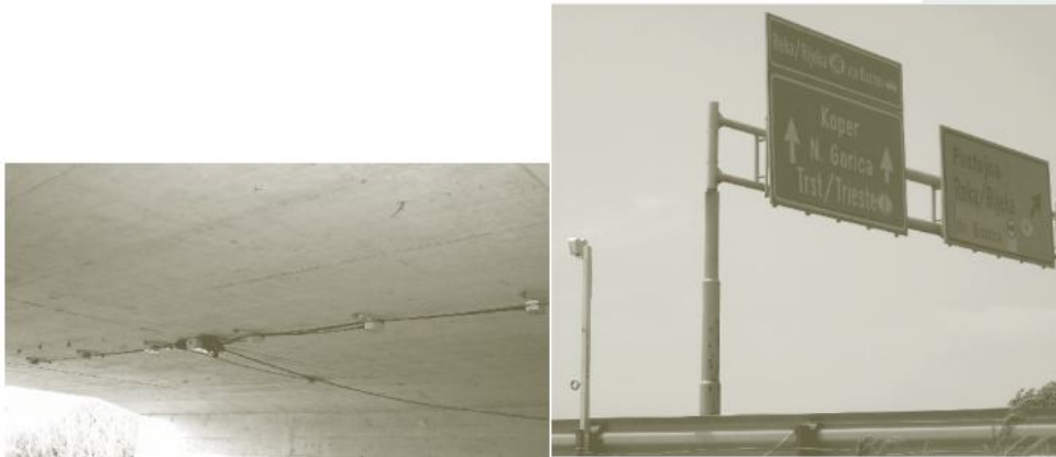
Slovenia bridge WIM System (source Commercial Motor Vehicle Size and Weight Enforcement in Europe)
